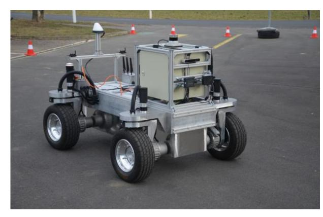
Autonomous robot to assess the performance, **safety**, and security capabilities of the RISC-V **multicore** platform.
